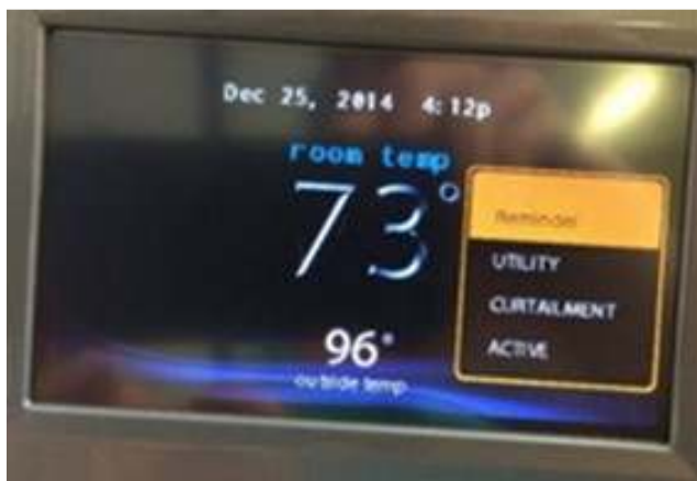
FIGURE 38. LABORATORY DR ASSESSMENT: UNIT CONTROLLER CONFIRMATION OF DR EVENT – VC SYSTEM 2
