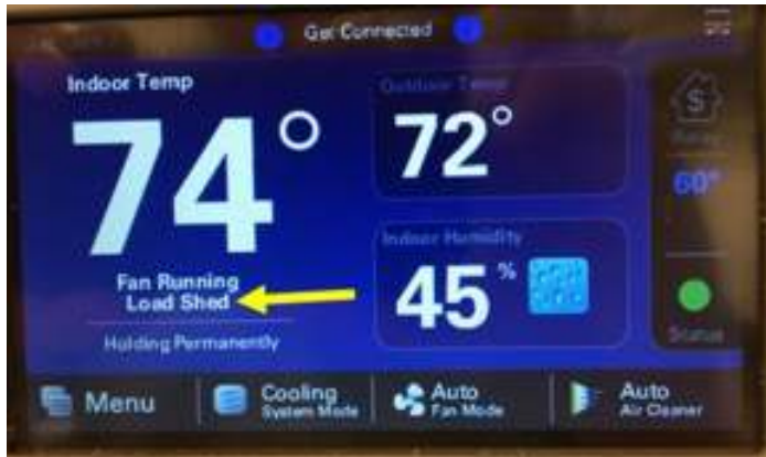
FIGURE 47. LABORATORY DR ASSESSMENT: UNIT CONTROLLER CONFIRMATION OF DR EVENT – VC SYSTEM 3
