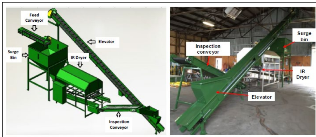
Figure 6: Components of pilot IR dryer [4]
