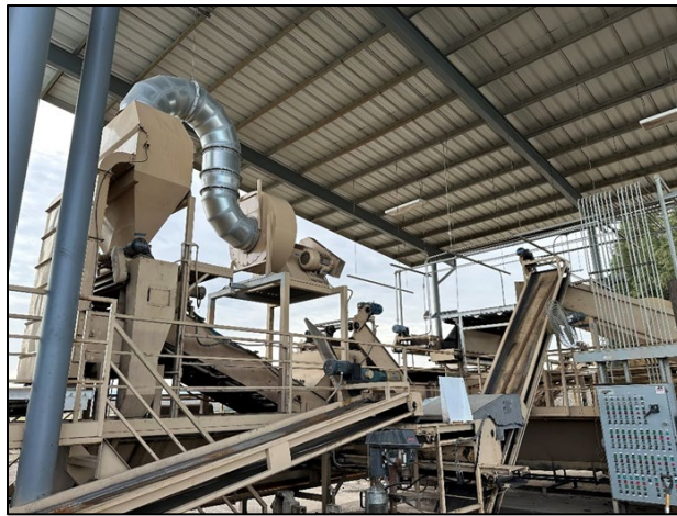
Figure 1: Waste removal, cleaning and dehulling of walnuts
