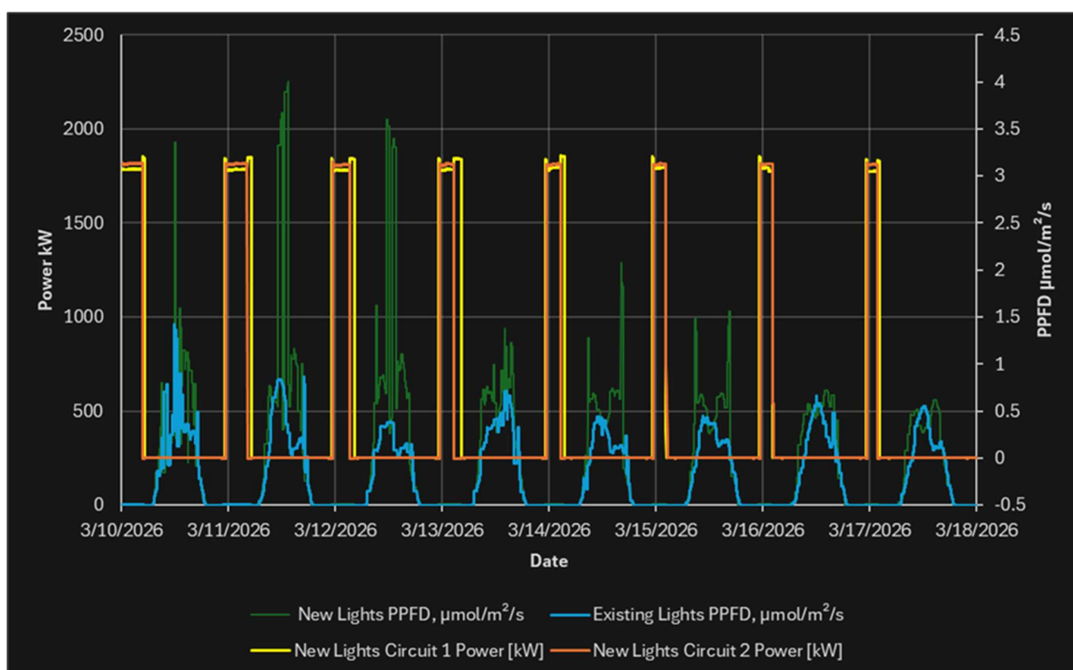
Figure 9: Lighting power and PPFD during "fully commissioned" period.
