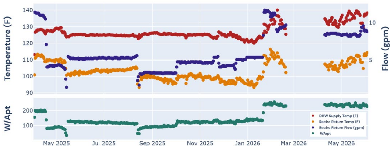
Figure 15: Increase in measured recirculation losses at Site 14 after crossover event.
