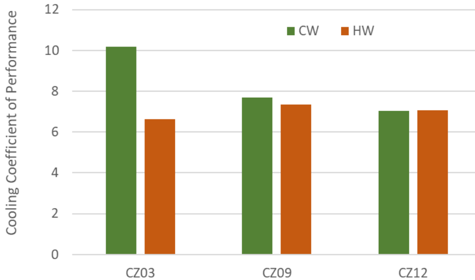
Figure 43: Cooling COPc condenser water vs. hot water – intermediate tank with 0-ton baseload.
