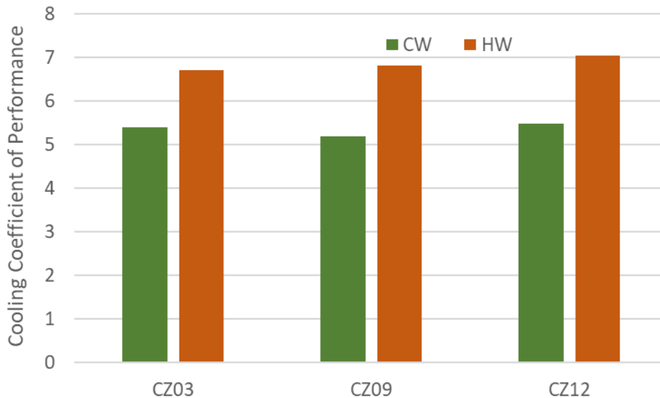
Figure 47: Heating COPh condenser water vs. hot water – intermediate tank with 50-ton baseload.
