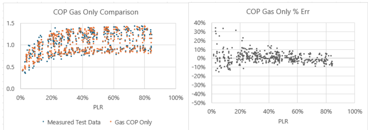
Figure 19: COP g comparison and error between model prediction data and measured data [3].
