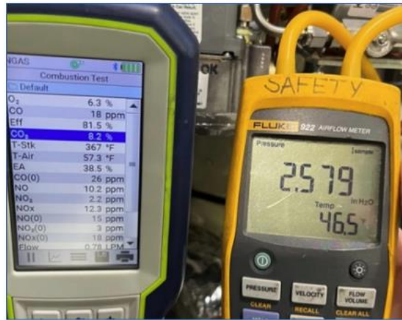
Figure 21: Exhaust gas constituents [left] and manifold pressure [right] [3].
