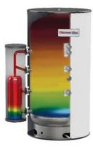
Tank stratification is advantageous for preheat GAHP systems. In a stratified tank, the hottest water resides at the top, allowing it to be delivered to the existing storage tanks. Meanwhile, the GAHP heat exchange coils can be positioned at the bottom, where the cooler water is located, ensuring that the coldest water is heated by the GAHP.
