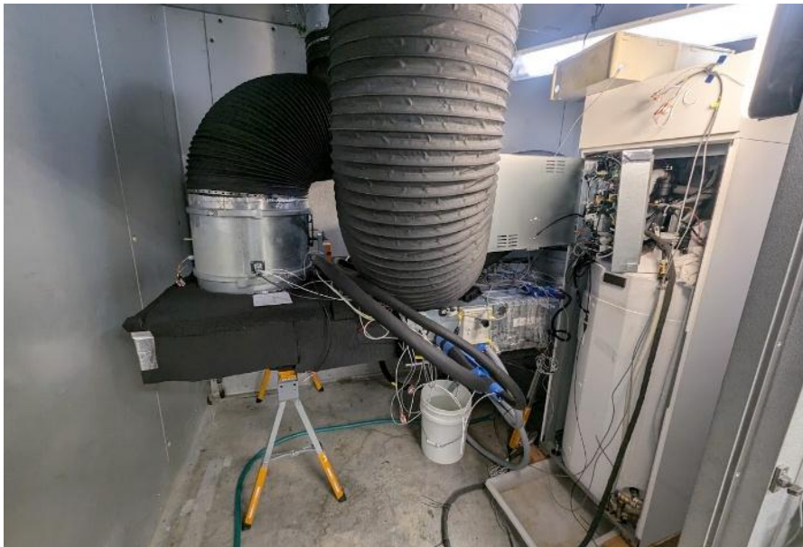
Figure 7: Variable-speed MFHP air handler unit (back horizontal grey section) and domestic hot water tank (front right with front cover off and white insulation visible) installed and instrumented in the indoor chamber.
