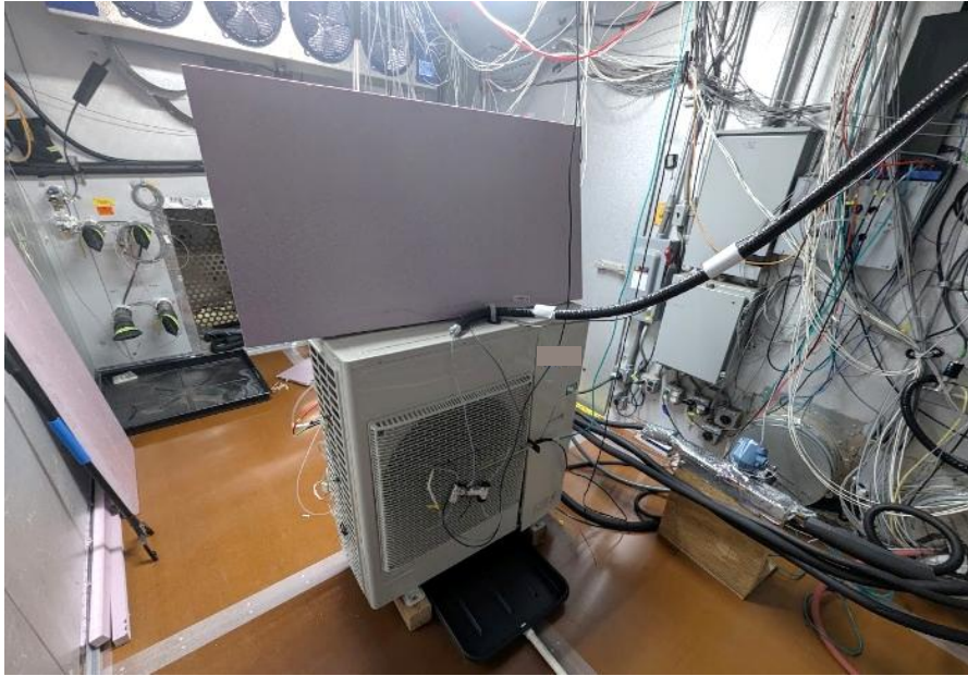
Figure 6: Variable-speed MFHP outdoor unit installed and instrumented in the outdoor chamber, ODU exhaust side visible.
