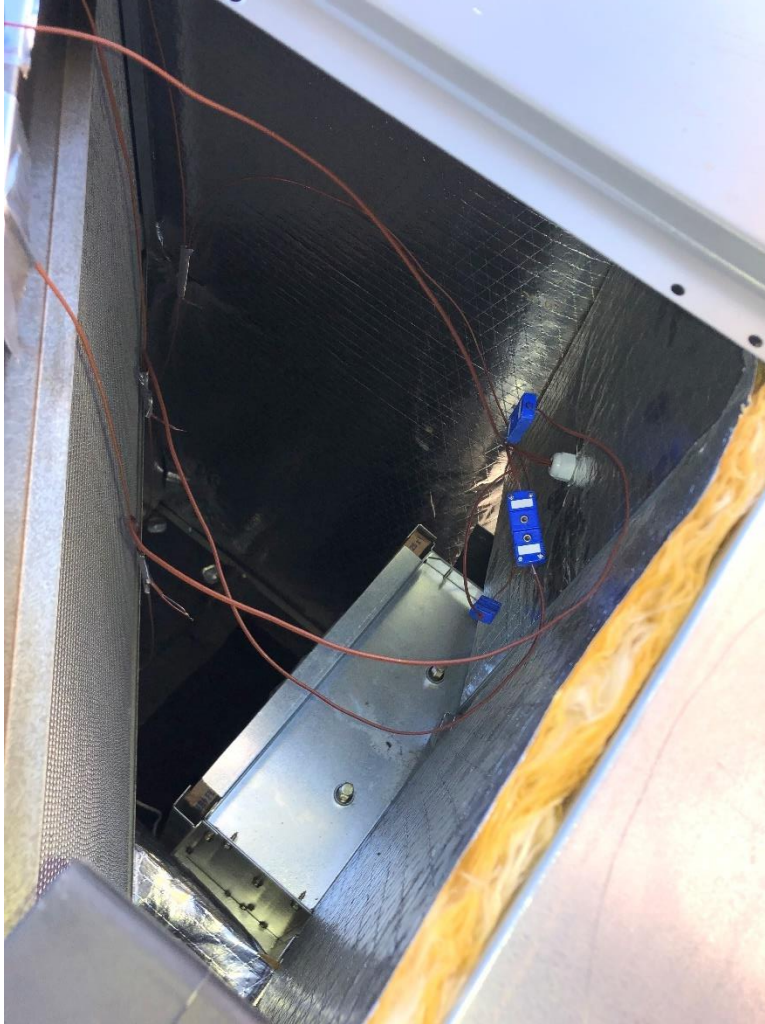
Figure 11: Mixed air plenum before the coil of the single speed HP RTU showing distributed thermocouples. (Temperature and humidity probe was also installed but not shown here)
