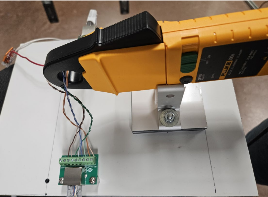
Figure 4: Fluke CT with Ethernet cable conductors passed through.
