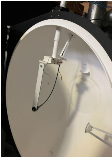
Figure 15: Unilluminated fiber in 1-meter integrating sphere.
