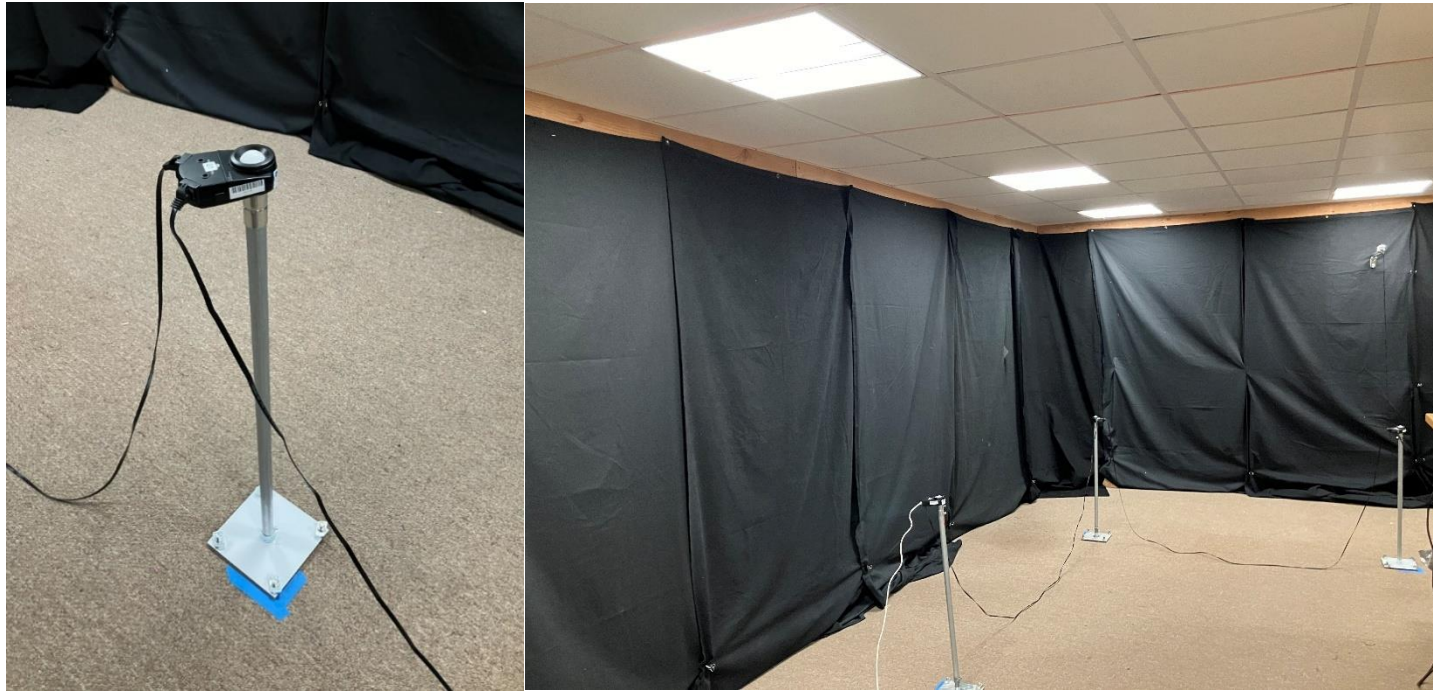
Figure 13: Work plane illuminance sensor.
