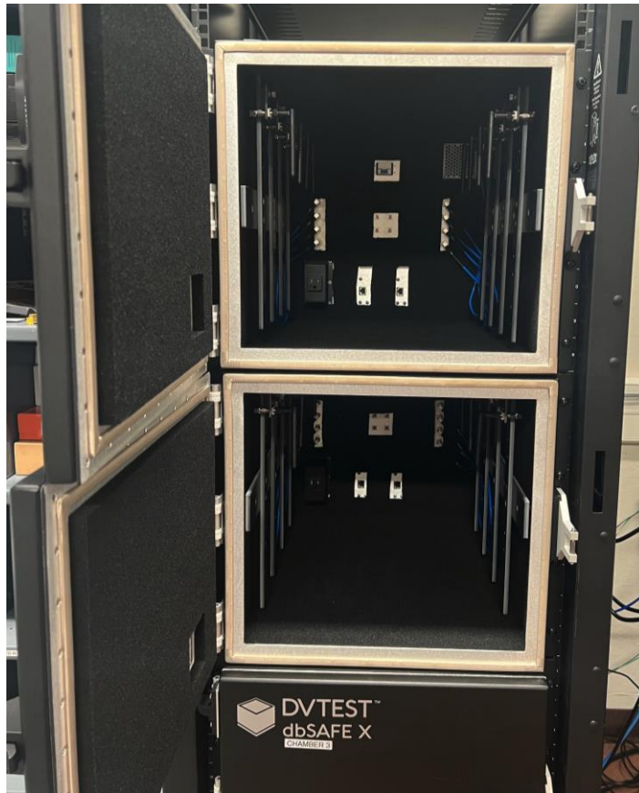
Figure 4: Anechoic chamber with attenuation antennas mounted
