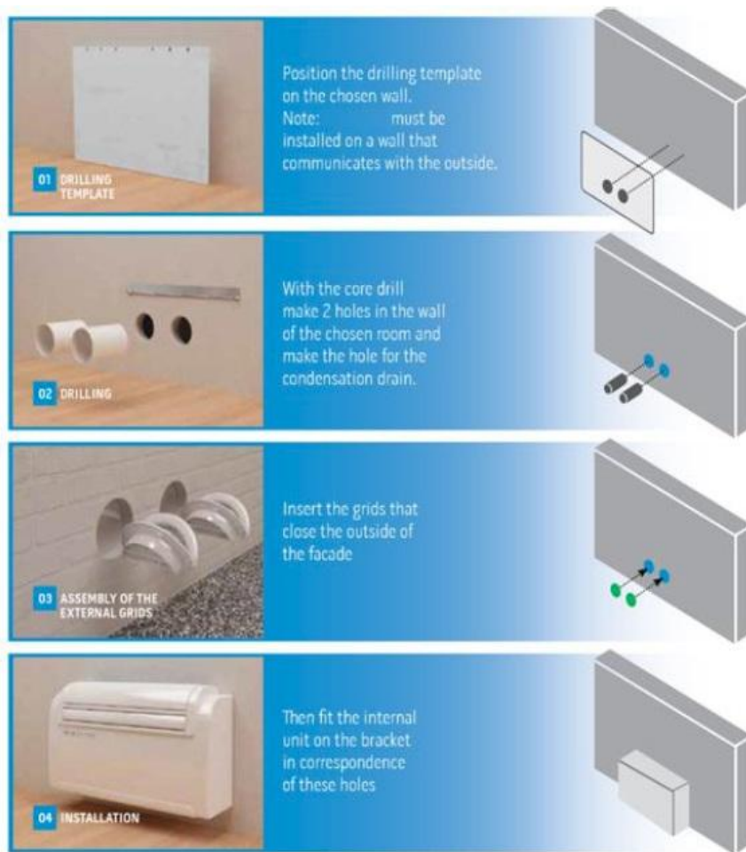
Figure 7: DDPHP installation process.
