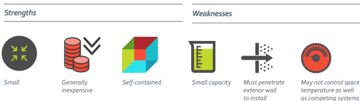
Figure 3: PTHP and PTAC design strengths and weaknesses.
