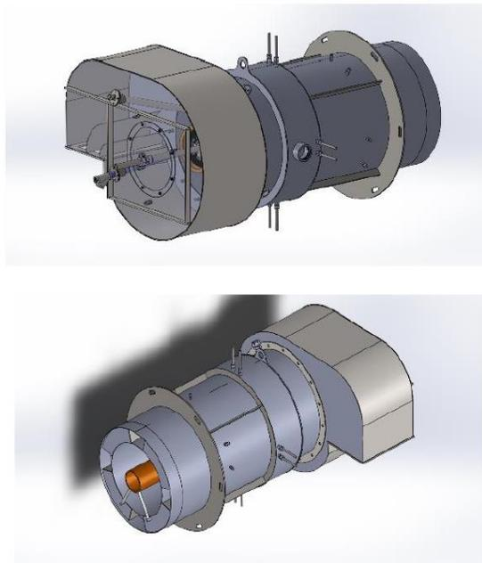
Altex has tested this burner in a firetube boiler setting, where NOx levels of 5.7 ppm were achieved, and corrected CO emissions were under 10 ppm. The successful operation of this burner led to the conclusion that the NZNB burner can be commercialized to meet stricter air quality regulations in California for boilers, water and process heaters.
