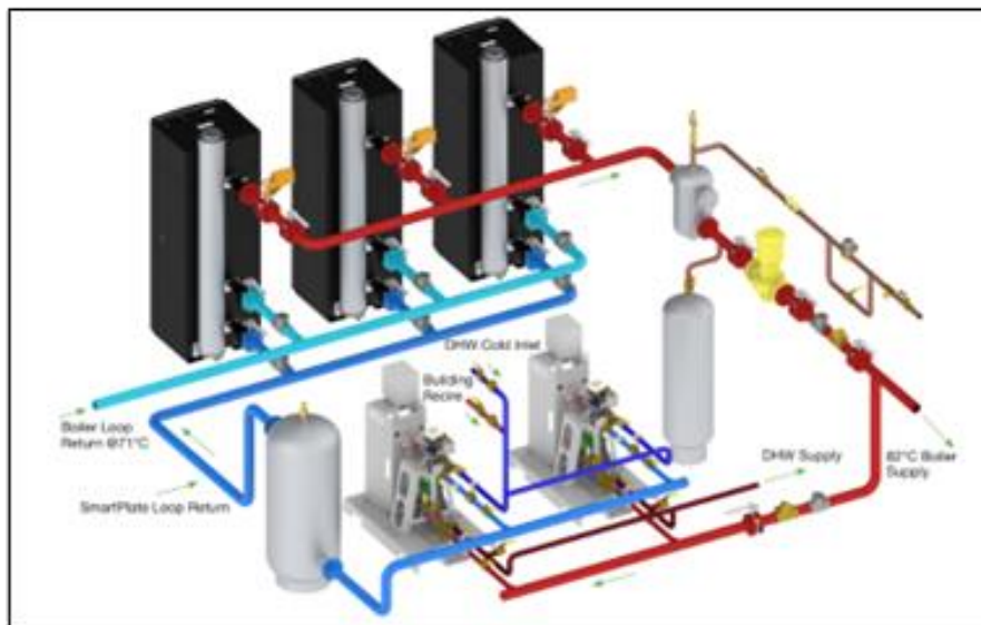
Figure 33: Combination plant with dual returns (Manufacturer I) [23]
