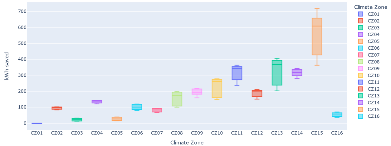
Figure 32. Cooling energy savings (one-story model, mid-COP, 86 °F setpoint).
