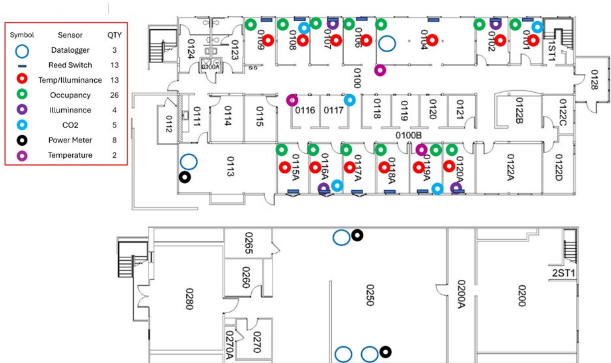
Figure 24. Layout of The Barn, showing locations of M&V sensors.
