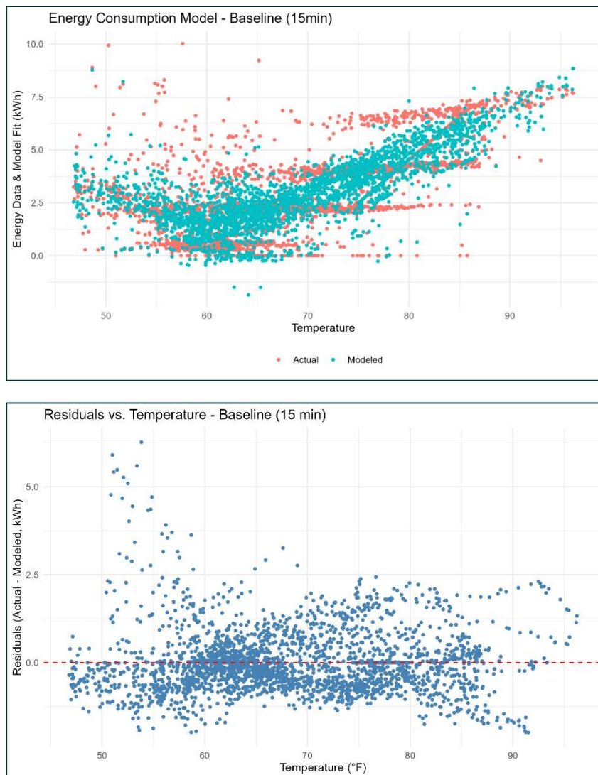
Figure 67: Measured energy vs. model-predicted energy for Baseline conditions vs. OAT (top) and Residuals
