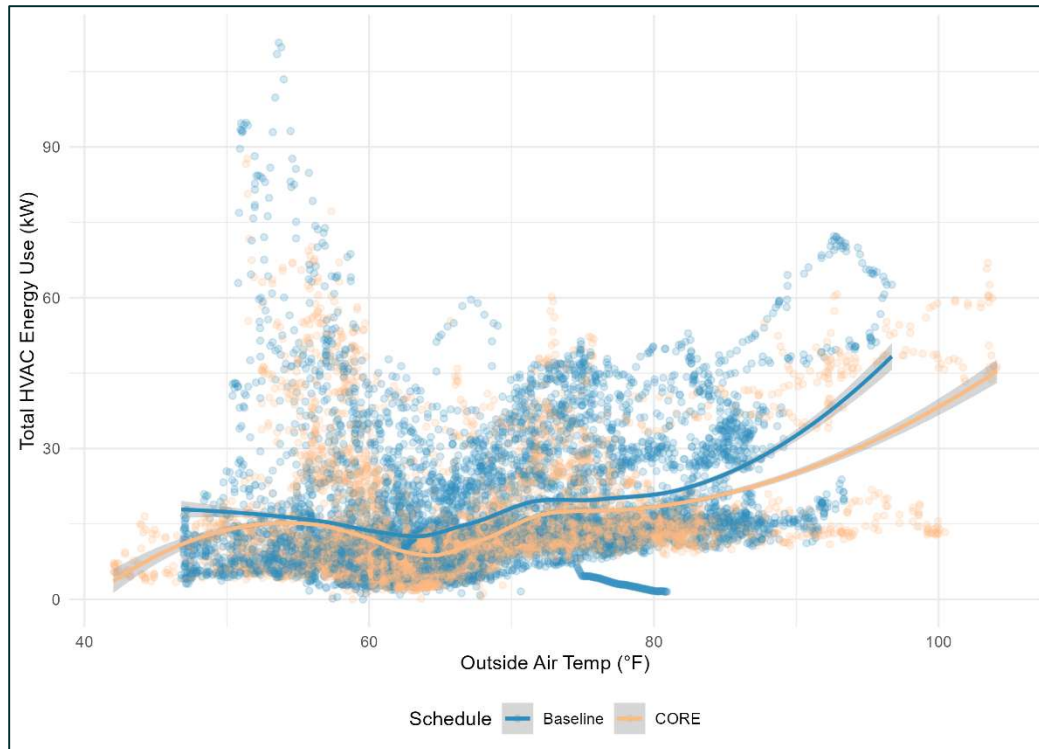
Figure 55: HVAC heating, cooling, and fan energy consumption vs. OAT for combined AHU 1 and AHU 2—MOB-3.
