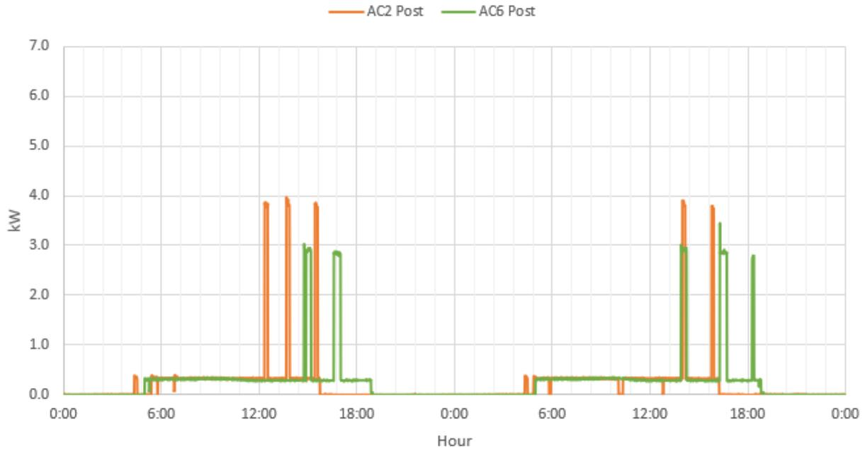
**Figure 18: The operating profiles of AC2 and AC6 on relatively hot days.**
