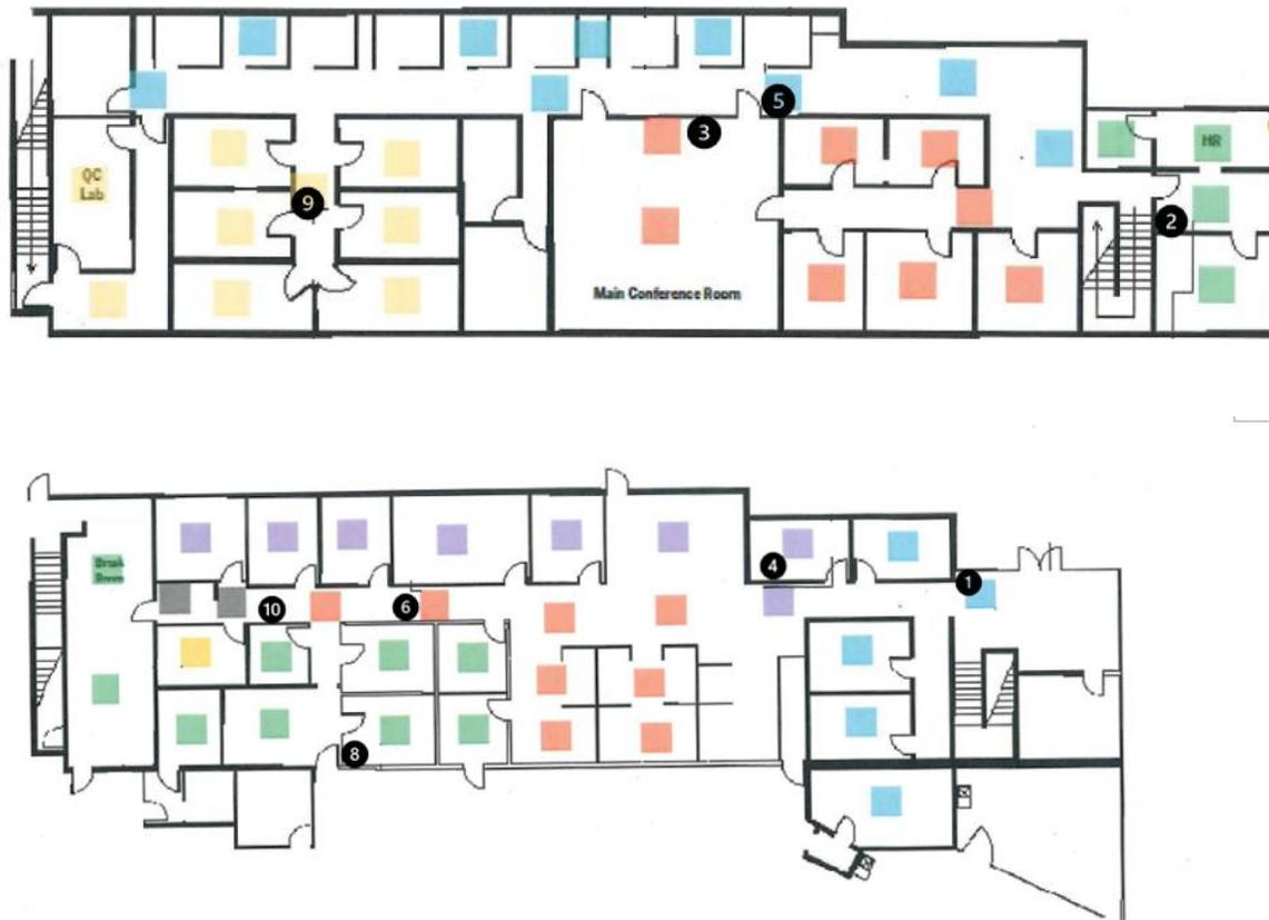
**Figure 10: Office layout (upstairs above and downstairs below) and the location of thermostats at Vista site**
