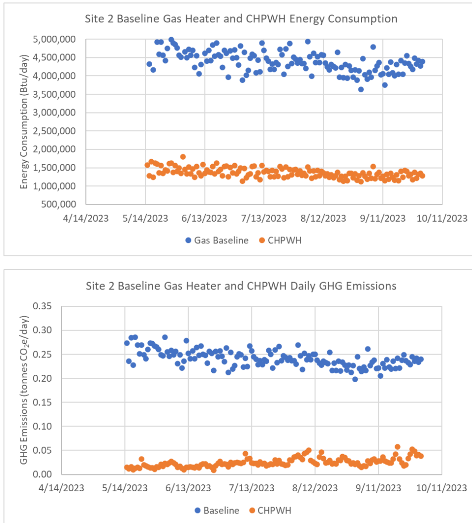
Figure 10: Daily baseline and CHPWH energy consumption and emissions over the monitoring period (Site 2).
