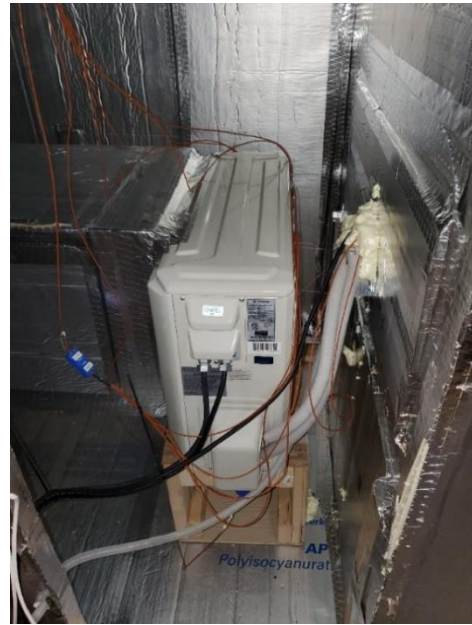
Figure 9. Baseline Unit in Test Chamber; Indoor and Outdoor Units During Installation (left), Outdoor Unit after Installation (right)
