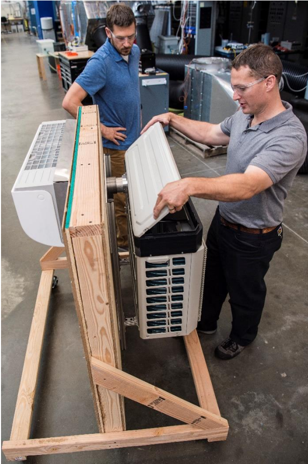
Figure 7. System Mounted on Demonstration Wall as in Actual Operation (left); Disassembled with Mounting Brackets (right)
