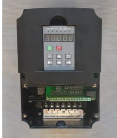
Figure 2: VFD internal wiring.
