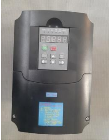
Figure 1: Variable frequency drive (VFD).
