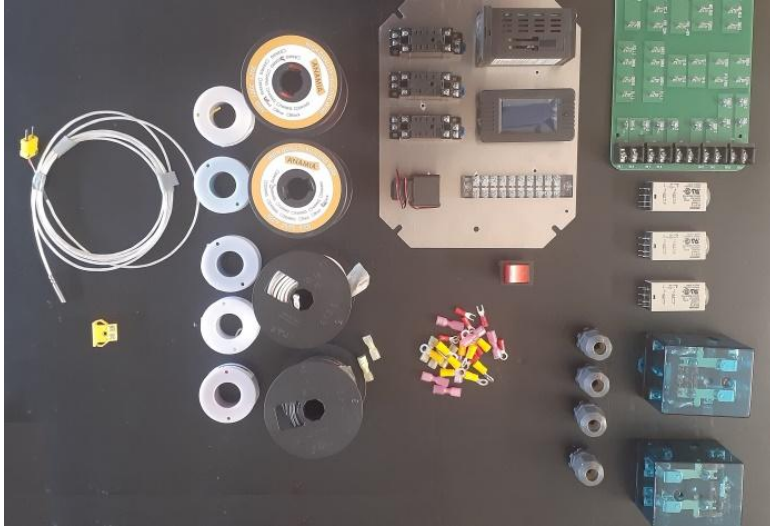
Figure 3: HVAC capacity controller components.
